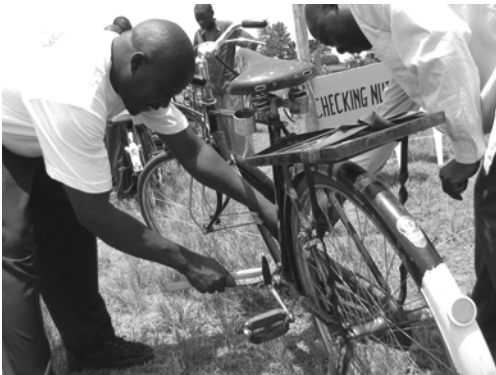
Figure 9. Repairing a cotted crank arm on a Hero bicycle. Hoima.
